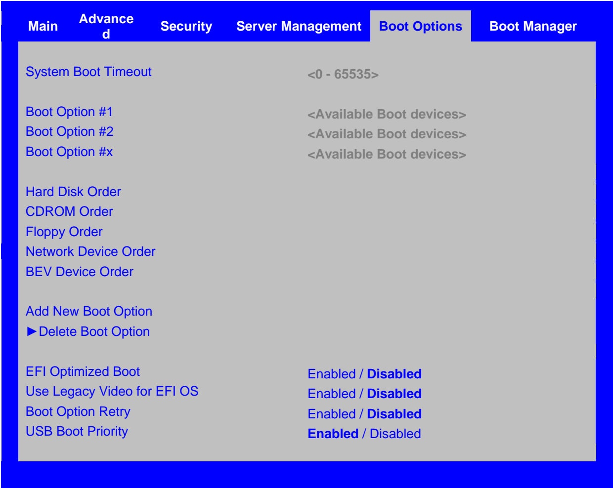
Figure 33. Setup Utility — Boot Options Screen Display
